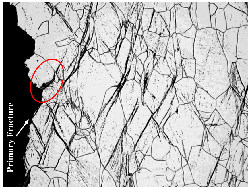
Figure 4. SIPH, primary fracture face, mid-wall. 200x.
